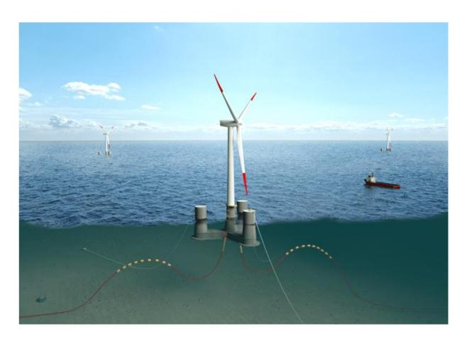
The American Bureau of Shipping (ABS) has issued Approval in Principle (AiP)<sup>1</sup> to the OO-STAR concrete semi-submersible floater from Bouygues Travaux Publics, a subsidiary of Bouygues Construction. It can support wind turbines of more than 20 MW in harsh offshore environments. This achievement is the first step in the
